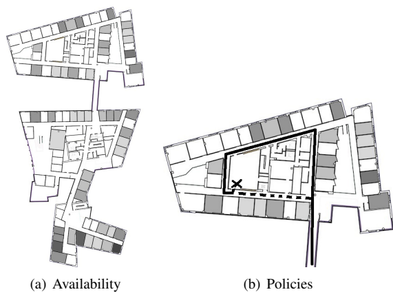
Fig. 3. (a) We measured the availability of humans in each of 78 offices in our building - darker gray represents higher availability. (b) The OPOMDP policy takes the shortest path to the lab (dashed line) while the optimal HOP-POMDP policy takes a longer route with more available people (solid).
