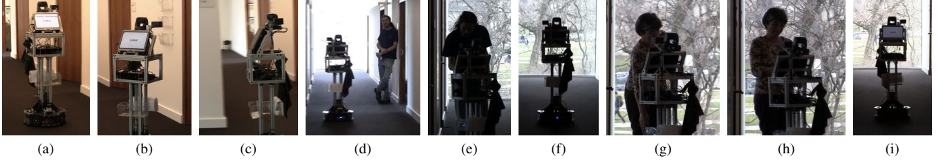
Fig. 3: (a,b,c) After CoBot-2 receives a Transport task request, it autonomously navigates to the location l_p to pick up a bottle of water and take it to location l_d . (d,e) Upon arriving to l_p , CoBot-2, asks a person to place the bottle of water and afterwards press ‘Done’. (f,g) Then, CoBot-2 navigates to location l_d to deliver the bottle of water. (h,i) When the user presses ‘Done’, CoBot-2 navigates back to its home location. (The complete video is submitted with this paper.)
